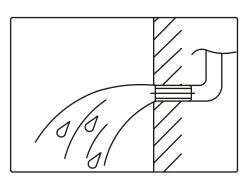
In order to avoid the obstruction of faucet, must to clean the impurigities and sludge of pipe, before assembly.
