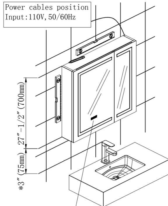
1). Determine the installation position of the LED Medicine Cabinet and mark it with a level on the wall.
