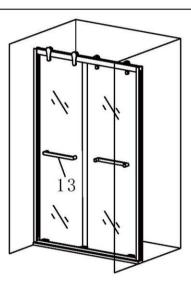
Install the handle of the movable door. Attention to the direction of the handle. Make sure the outside handle rod is out, and the inside handle rod is in.
