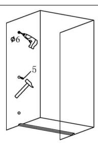
Measure the side column horizontally by spirit level, make the fixing screw hole position by pencil, remove the down rail and side colume, drill a hole and and insert with plastic expansion screw.
