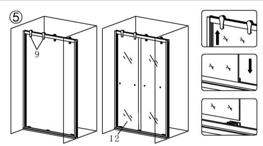
Put the sliding wheel to the up rail, remove the moveable glass, and insert the buttom of the moveable glass to the sliding cover.
