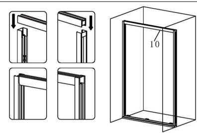
Make the both ends of the uppper rail into the slot of the side column, push down hard to make it flatten. After install the up-rail, adjust the length of both ends, so that the length of which rail of the column is the same.
