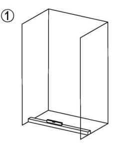
Select the installation position, put the tray or base stone to the position and measure it horizontally by spirit level.
