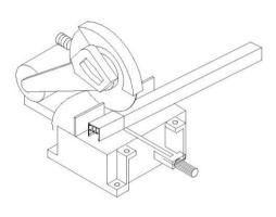
Cut the Top Guide Rail -10mm shorter than the top dimension W1.
