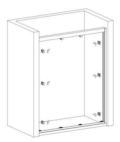
Install anti-collision rubber.
