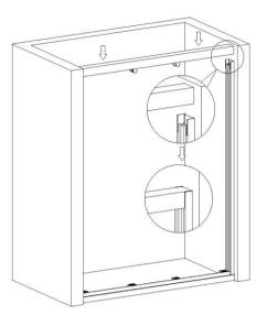
Put the both ends of the top guide rail to the left and right side column.
