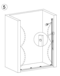
Lock the left and right side column tightly by a ST4 $\times$ 30 tapping screw.
