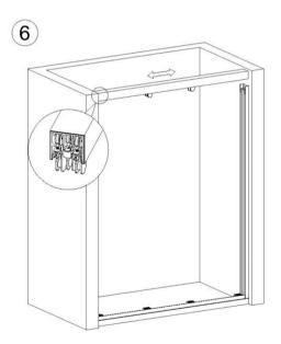
Adjust the up-rail to make the space between the left and right side column is the same.
