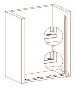
Insert the left and right side column to the bottom guide rail.
