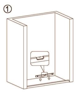
Select the installation position, put the tray or stone base to the position and measure it horizontally by spirit level.
