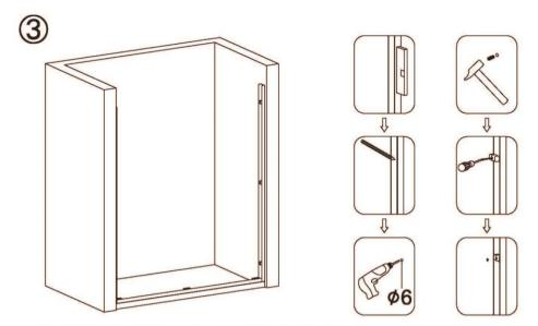
Measure the side column to make it vertically by spirit level, make the fixing screw position, drill a hole of  $\phi$ 6, strike the plastic inflatable glue through anti-collision rubber and fix the side column to the wall by ST4×45 tapping screw.
