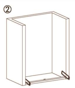
If the down-rail is too long, it's will be saw cutted. Measure and make the cutting part into two same dimensions and cut it smoothly.
