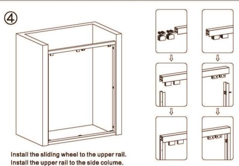
Adjust the length of both end of the upper and down sliding rail, make the right and left the side column the same length.
