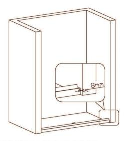
Put the down-rail to the installation position, make sure the down-rail is in the middle position, leave 8mm space at both end to install side column.
