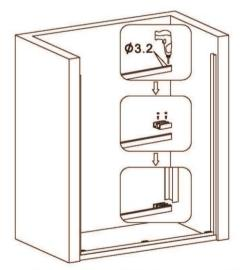
Mark the fixing screw position of the sliding wheel, and drill a hole of \$\phi 3.2\$. Fix the sliding wheel to the down-rail by M4×12 tapping screw, install decorative cover.
