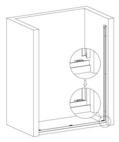
Insert the left and right side column to the bottom guide rail.
