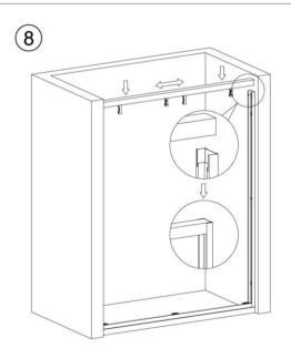
Put the both ends of the top guide rail to the left and right side column. Adjust the up-rail to make the space between the left and right side column is the same.
