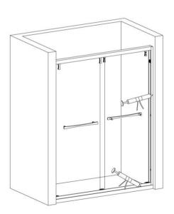
Finally seal with glass glue around the shower room. It can be used after 24 hours.
