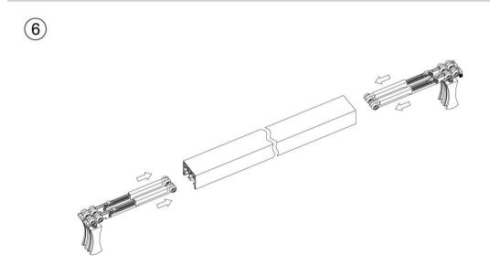
Put the damping wheel to the top guide rail.
