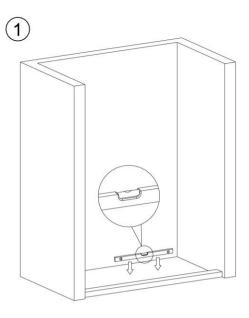
Measure by spirit level, adjust to make sure the installed position is horizontal.
