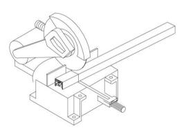
Cut the Top Guide Rail -8mm shorter than the top dimension W1.
