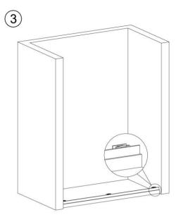
Put the bottom guide rail to the installation position. Make sure that bottom guide rail is in the center position, leave some space at both ends in order to install side column.
