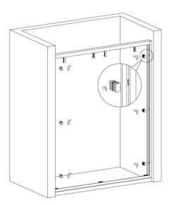
Install anti-collision rubber.
