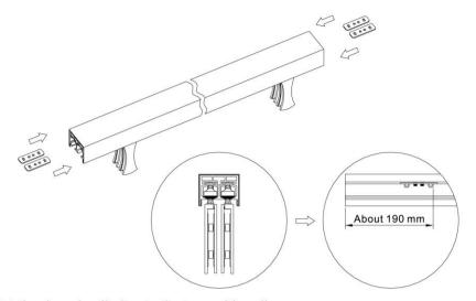
Put the damping limiter to the top guide rail. Adjust the distance from position to the edge, about 190 mm, loked it tightly by a 2.5 mm hexagonal key.
