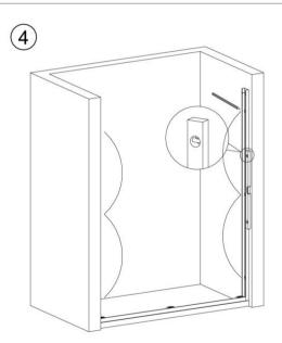
Ensure the water material is vertical, make a hole by pencil.
