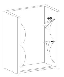
Drill a hole by an  $\phi$ 6 driller, Knock in the 6mm expansion screw.
