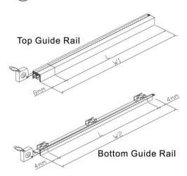
The Top Guide Rail can be cut from either end.
