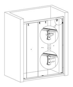
Adjust the high-low and verticality of the moving glass by spanner twisting the hexagonal screw, then put on the decorative cover.
