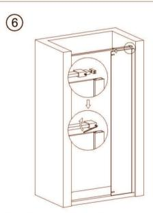
Install the draw bar parts. Tight the tube seat with a 3 mm hexagonal key.
