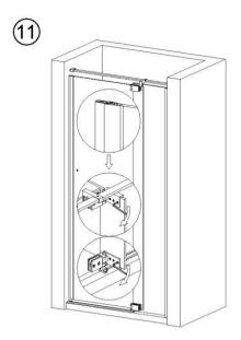
Adjust the moving glass, make sure the magnetic stripe adsorbed tightly.
