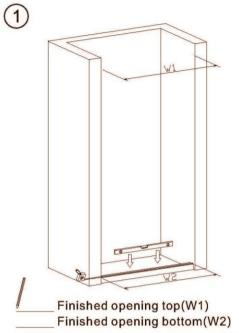
Measure by spirit level, adjust to make sure the installed position is horizontal.
