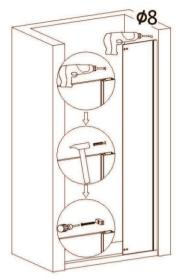
Drill a Ø8 hole. Knock in the Ø8 Rubber. Lock the tube fixing part tightly by a ST5×35 tapping screw.
