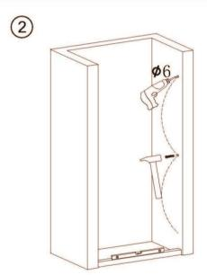
Drill a hole by an **Ø**6 driller, Knock in the 6mm expansion screw.
