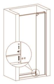
Drill a **6** hole. Knock in the **6** Rubber. Lock the rubber waterproof bar tightly by a ST4×30 tapping screw.
