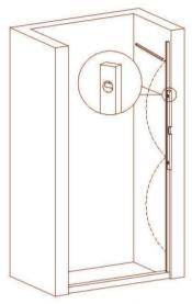
Ensure the water material is vertical, make a hole by pencil.
